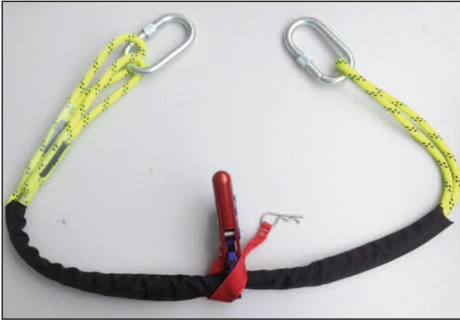
Step 3: Fit Quick Release and Karabiners (4t) ▲
