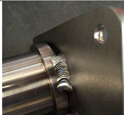
Fig 1.2: CB2723-Issue E Modified Bracket (additional external weld visible)
