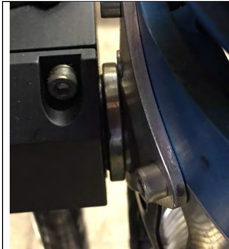
Fig 1.1: CB2723-Issue A to D Original Bracket (no external weld)
