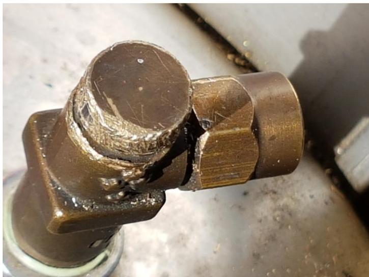
Fig 1. FLLG damaged by inappropriate use of tools.
