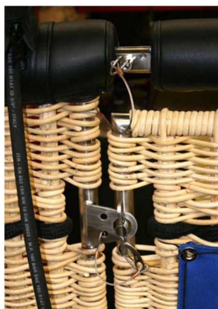
FIG S5-4 Top bar release pin installed, upper door latch secured and safety hook attached.
