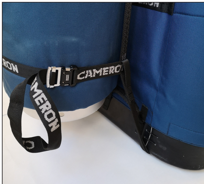
▲ Correct rigging of lower cylinder strap
