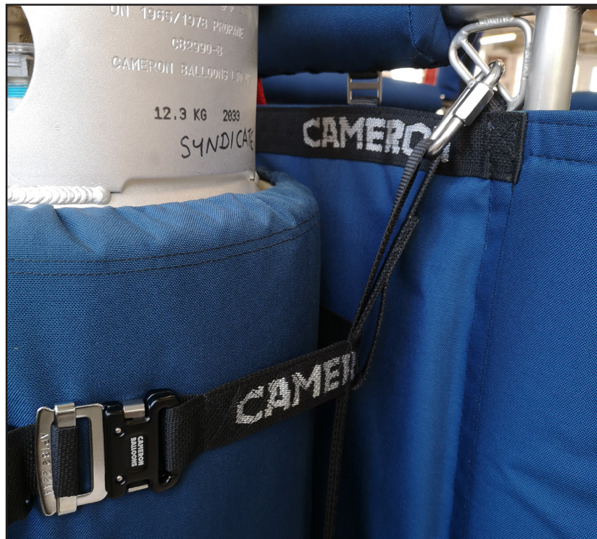
▲ Correct rigging of upper cylinder strap
