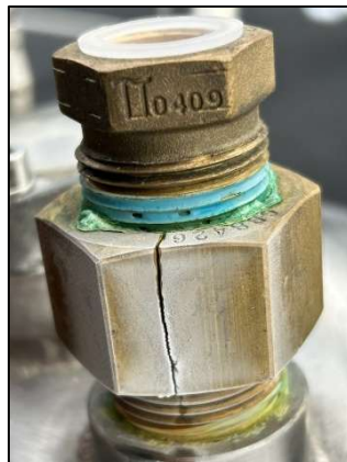
Figure 2 - Cracked CB8426, PRV Adaptor
