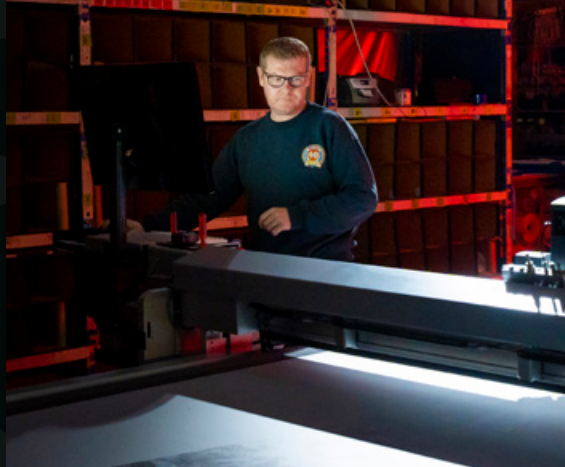
▲ THE PLOTTER CUTTING FABRIC INTO GORES
